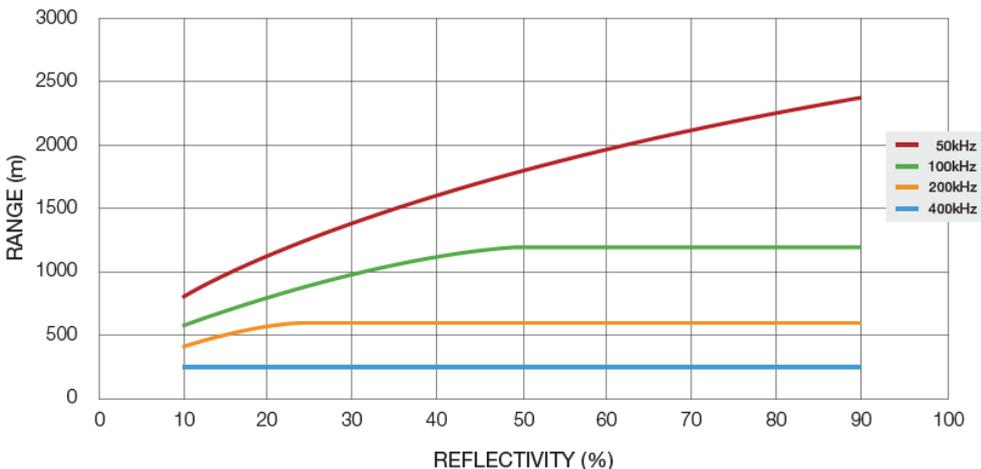
Figure 1 Graph of reflectivity versus distance range in meters (Sentry Field Operator Manual).
