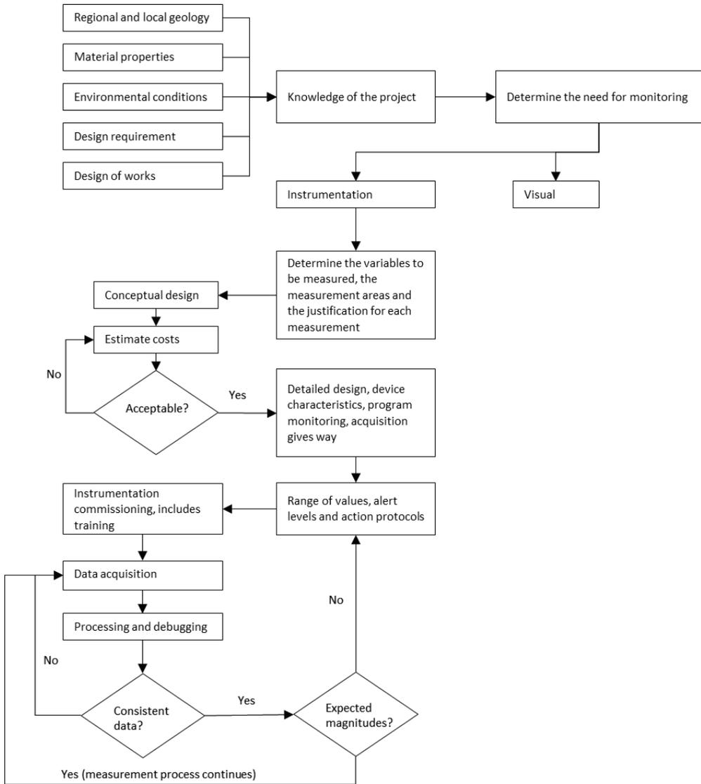
Figure 2 Sequential diagram for implementing instrumental monitoring.
