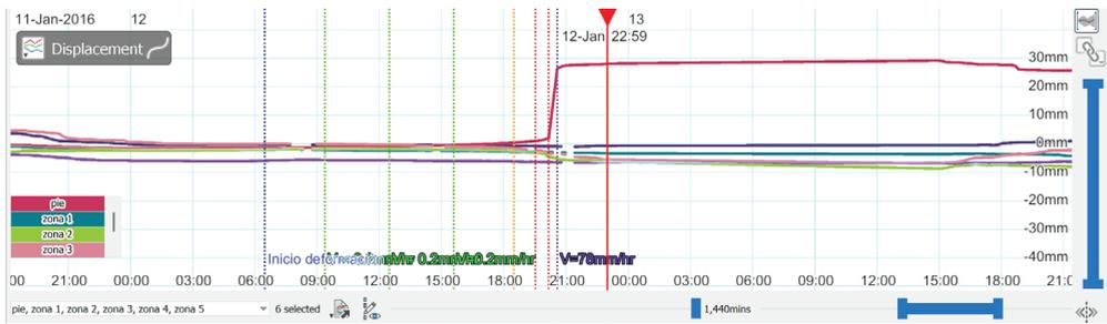
Figure 6 Monitoring zone, Tailings dam wall with color legend by displacement. Date: January 12, 10:59 p.m.
