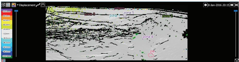
Figure 4 Monitoring zone, Tailings dam wall with color legend by displacement. Date: January 8, 8:15 p.m.
