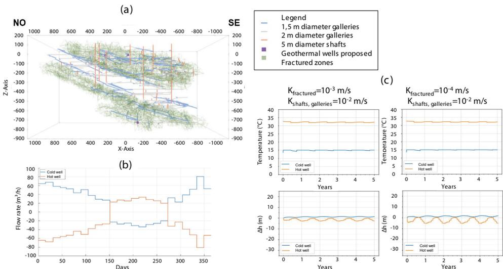
Figure 6 (a): Representation of the mine reservoir. (b): Example of demand flow profiles. (c): Resulting simulated production temperature and head variations at the two wells of the system over a 5-year period for defined hydraulic properties of existing shafts and galleries of the mine reservoir and of fractured zones resulting from coal exploitation.
