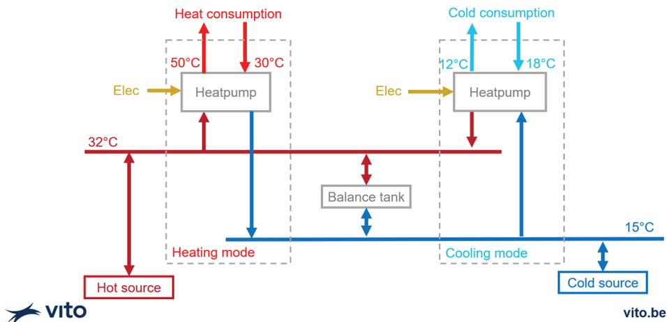
Figure 4 Conceptual design of the investigated mine water geothermal system, called GEOMINE system.
