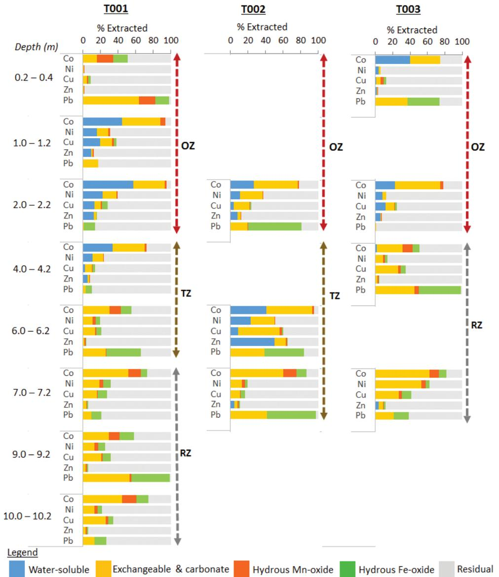
Figure 3 Results of the SEPs performed on TD materials with depth. Depths shown are consistent across T001, T002 and T003 but are not shown to scale downhole to conserve space.
