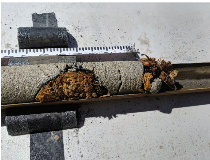
Figure 4 Core Sample Covered from Verification Drilling. Note that the Grout Material has Flowed Around and Completely Infilled the Space Surrounding a Wooden Support from the Mine
