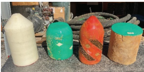
Figure 9 "Pigs" that are used to push through pressurized line to clean the line (image: Greg Phillips)
