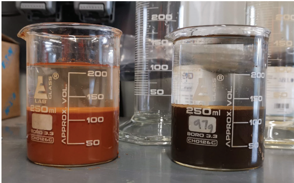
Figure 4 Sludge produced during pilot trails, Iron / Arsenic Stage II sludge on the left and Manganese Stage IV sludge on the right.
