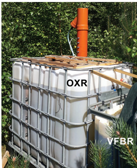
Figure 2 Arrangement of OXR and VFBR in the field (left) and a sketch of the vertical tube principle according to Torricelli's theorem for adjusting the flow of the OXR feed
