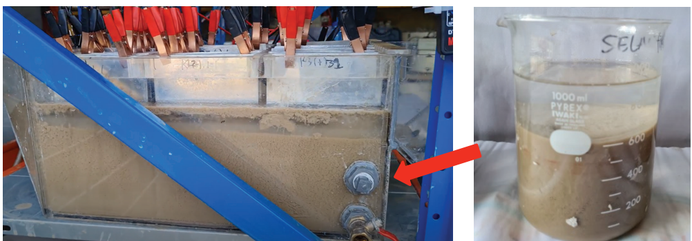
Figure 5 Continuous Electrocoagulation Experiment (a) dead zones in reactor (b) Electrocoagulation after 60 min of settling time in 16.3 A/m 2 - 0.3 L/min
