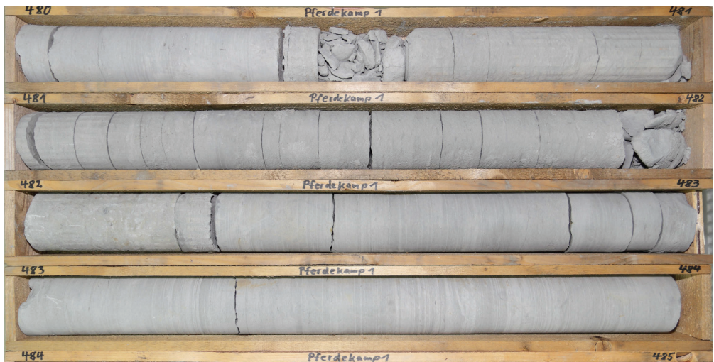
Figure 2 Core barrel from the monitoring well “Pferdekamp 1”, depth 480–485 m, showing Emscher Formation marls (GD NRW 2022)
