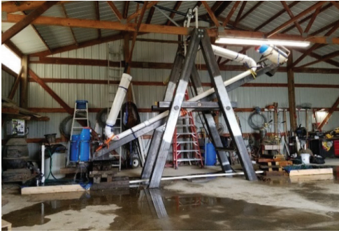
Figure 1 14 ft MT Water Motor without attachment operating
