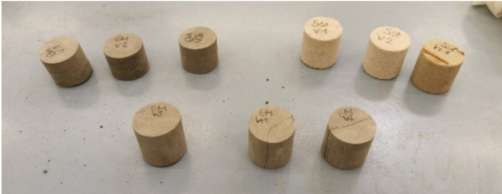
Figure 1 Plug samples from the Emscher Marl and Bentheim Sandstone (image: Lisa Rose).
