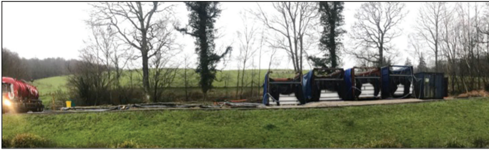
Figure 8 Passive Treatment Pilot Plant from right to left (Feed Tank; BCR1, 2, 3, 4; Reed bed (APW) 1, 2, discharge holding pond showing purple/white bacteria).
