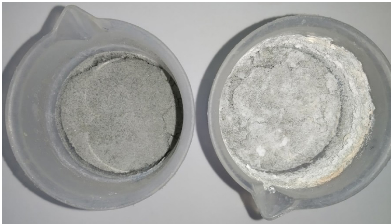
Figure 1 Appearance of the loparite ore concentration tailings at the end of the experiment. From left to right: moisturizing agent – distilled water, sulfuric acid solution.
