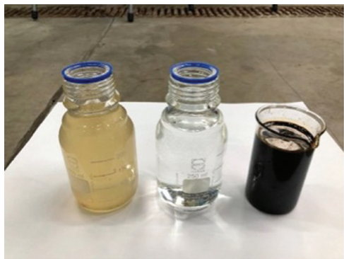
Figure 3 Oil and salt containing produced water before (left side) resp. after (center) Osmodialysis and oil fraction separated from it (right side).
