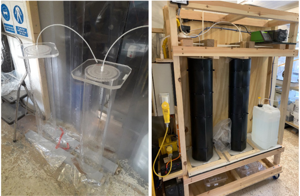
Figure 1 Laboratory columns and set-up (image: Geochemic Ltd).
