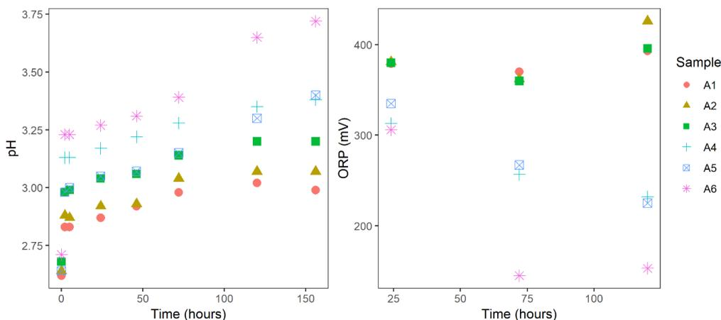
Figure 3 pH change and Redox potential for dilutions of coal mine ARD contacted with 25g of Sugarcane Bagasse
