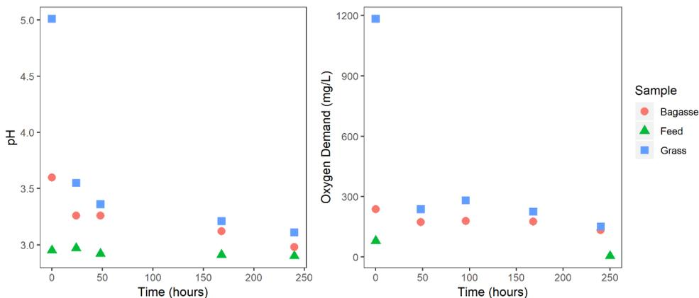
Figure 4 pH and Chemical Oxygen Demand at the outlet of pre-treatment reactor pairs filled with 200g of Bagasse and Grass respectively, on contact with ARD at a flowrate of 0.8L/day
