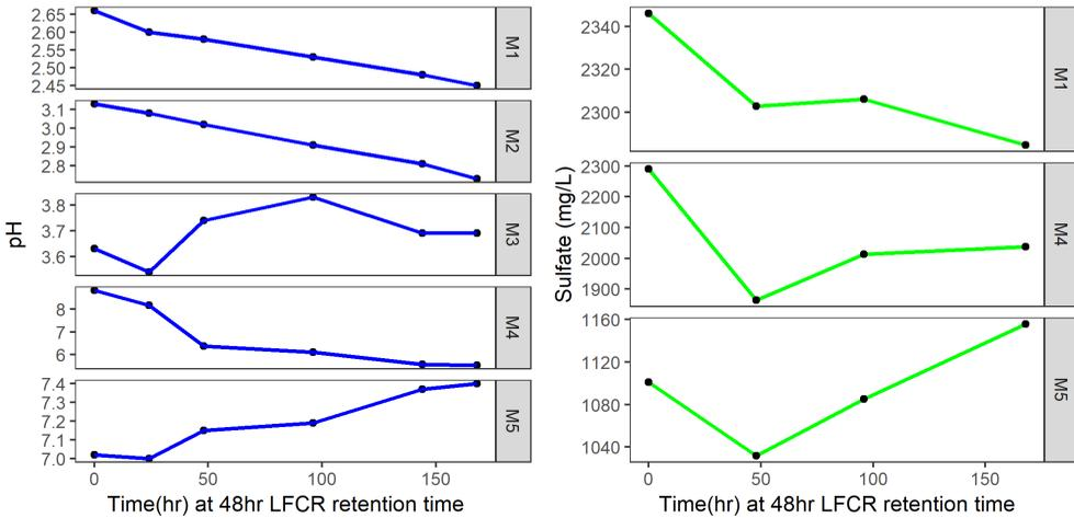
Figure 5 pH and Sulfate concentration for the model continuous flow system as shown in Figure 1 with a 48hr hydraulic retention time
