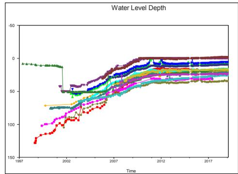
Figure 3 Water level time graph of the mine groundwater regime
