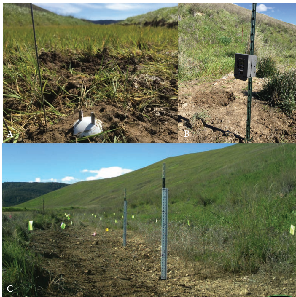
Figure 1 A) Inundation sensor, B) camera installed on t-post for flow-imagery monitoring, C) sample flow-imagery image, including flagging.
