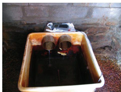
Figure 3 – Image of the ochre products in the study area. Crustification of surface drainage channels (left); Deposition of fluffy precipitates in the pipes, associated with the long term passage of the water (right).
