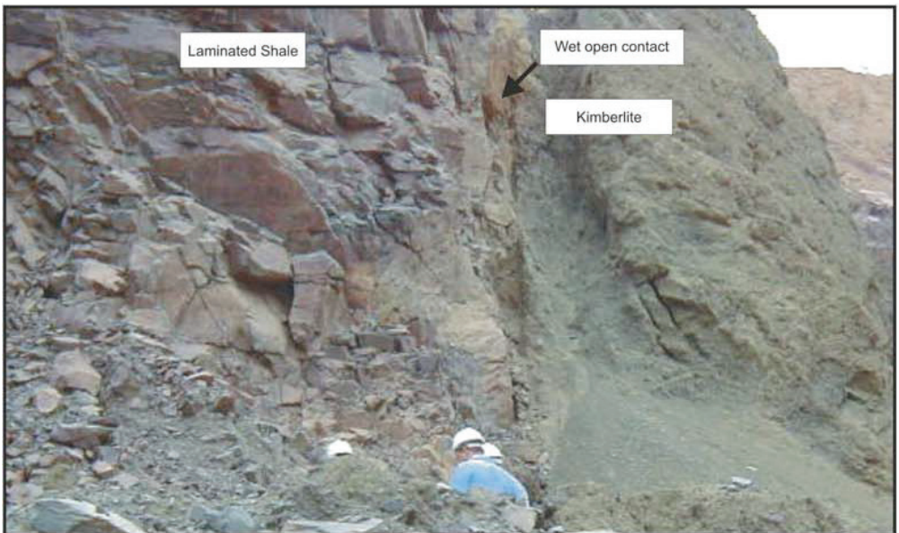
Figure 6 Jwaneng Mine Zone of Relaxation and wet kimberlite contact (crater)
