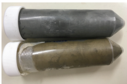
Figure 4. Subsamples of tailings from 77 m depth (grey, above) and 44 m depth (brown, below) showing the colour difference between the samples.
