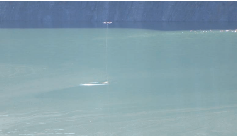
Figure 1 The Hatch drone aircraft sampling Pamour Pit, Ontario, Canada, June 2017
