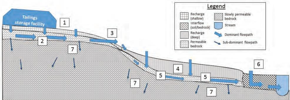
**Figure 1** Conceptual hydrological response model of hillslopes in Mine A.
