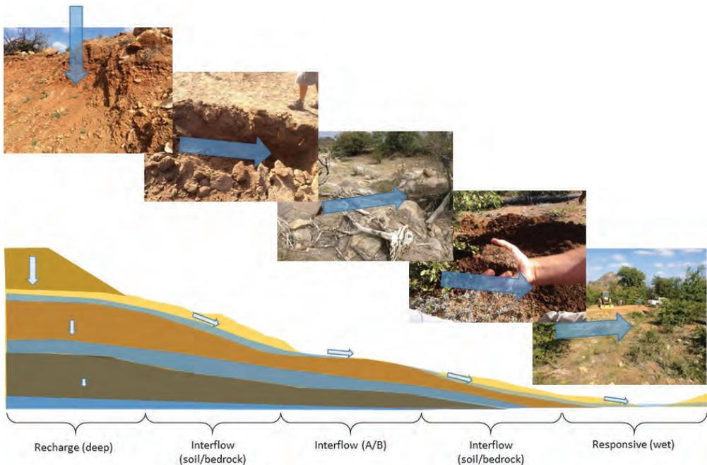
Figure 2 Soil distribution pattern and conceptual hydrological response model of hillslopes in Mine B.
