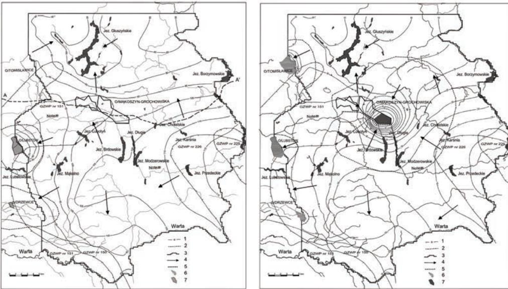
**Figure 4** Map of of hydroisohypses of the Neogene-Paleogene-Mesozoic aquifer a) in quasi-natural conditions, 2008 y, b) in hydrodynamic conditions for 2044 y, computer model prediction. Explanation: 1-piezometric surface of Neogene-Paleogene-Mesozoic aquifer, 2-range of the cone of depression, 3-model boundary, 4-groundwater flow direction, 5-hydrogeological cross-section, 6-mine drainage area, 6-pit lakes
