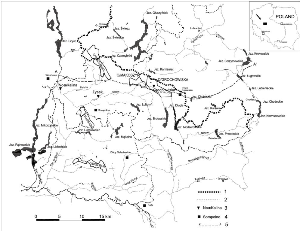
Figure 1 Hydrographic map of the „Mąkoszyn – Grochowska” lignite deposit area (modified from Stachy *ed.*, 1987). Explanations: 1- first order watershed, 2- other watersheds, 3- hydrometric station, 4- precipitation station, 5- hydrogeological
