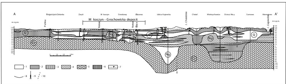
Figure 2 Hydrogeological cross-section (Szczepiński Straburzyńska-Janiszewska, 2011). Explanations: 1- fine sands, 2- glacial tills, 3- silts, 4- clays, 5- marls and dolomites, 6- lignite, 7- Neogene-Paleogene-Mesozoic aquifer piezometric surface, 8- stratigraphic boundary, 9- screeded intervals, 10- faults.
