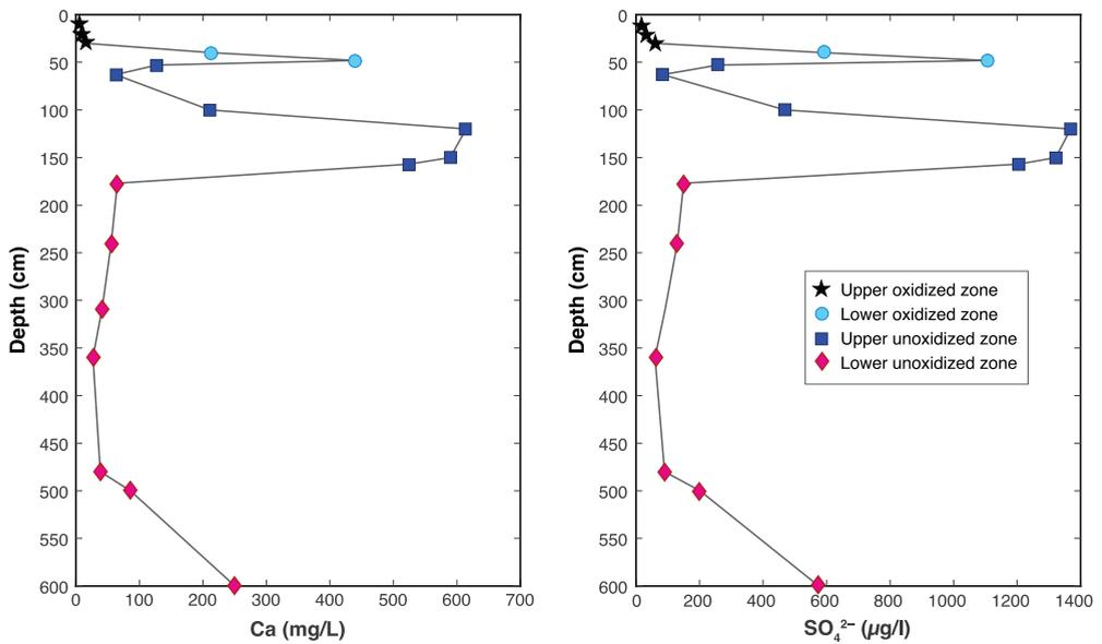
Figure 3: Ca and  $\text{SO}_4^{2-}$  distribution in leachates from the Yxsjöberg W-tailings deposit, Sweden.
