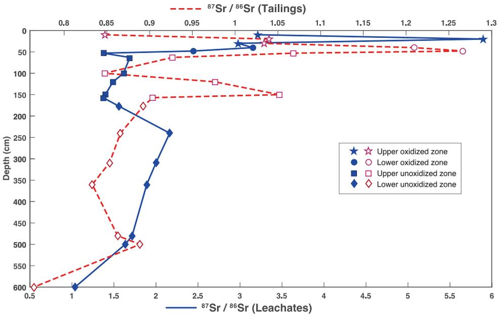
Figure 1: Sr isotopes ratios ( $^{87}\text{Sr}/^{86}\text{Sr}$ ) in leachates (—) and tailings (---) from Yxsjöberg mine site, Sweden. The  $^{87}\text{Sr}/^{86}\text{Sr}$  signatures at 600 cm depths represents a mixture of tailings and till and have been neglected in this study.
