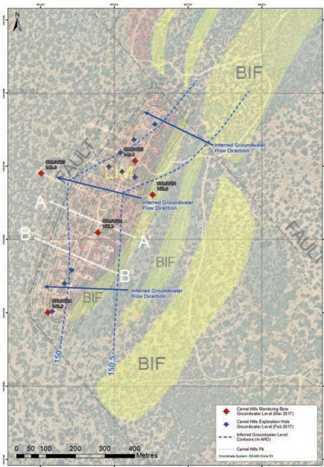
Figure 2 Site Geology, Groundwater Levels and Flow Directions
