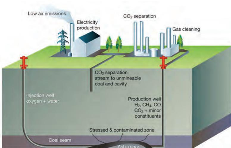
Figure 1 Depiction of underground coal gasification (Adapted from Burton et al, 2006)
