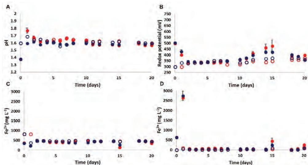
**Figure 2** A) pH, B) redox potential, C)  $\text{Fe}^{2+}$  and  $\text{Fe}^{3+}$  of the HS experimental (●) and LS experimental (●) and the HS control (○) and LS control (○) column PLS values over the course of the experimental period. Error bars represent the standard deviation from the mean pH across the experimental columns.
