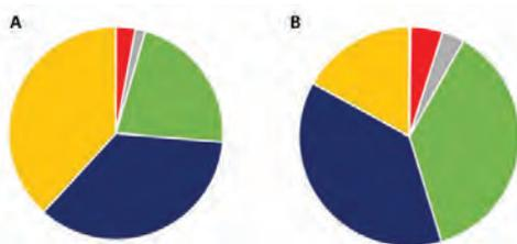
**Figure 1** Mineralogical analysis of the two waste rock samples acquired using QEMSCAN. A (PEL-HS) and B (PEL-LS) are results of the waste samples showing abundant acid forming minerals (pyrite and pyrrhotite;  $\odot$ ), dissolving mineral (calcite;  $\ominus$ ), fast- (garnet;  $\bullet$ ), intermediate- (Mn-Fe silicate and augite;  $\circ$ ) and slow-weathering (K-feldspar and muscovite;  $\circ$ ) respectively, and quartz as an inert mineral ( $\circ$ ).
