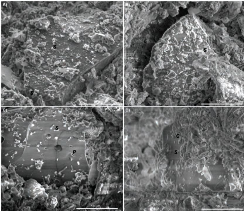
**Figure 3** SEM images of colonised pyrite bearing waste rock surfaces coated onto glass beads and leached over 20 days. Microbial mineral interactions on PEL-LS surfaces are shown in micrograph A (day 1, 18 hrs) and C (day 20) and interactions on PEL-HS surfaces are shown in micrograph B (day 1, 18 hrs) and D (day 20). Observed surface features including single cells (S), colonies (C) and pits (P), are labelled. A scale bar (10  $\mu\text{m}$ ) is shown on each image.
