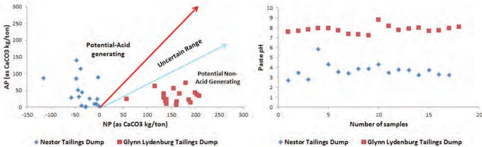
Fig. 2 Classification based on acid potential (AP), neutralising potential (NP) and paste pH.
