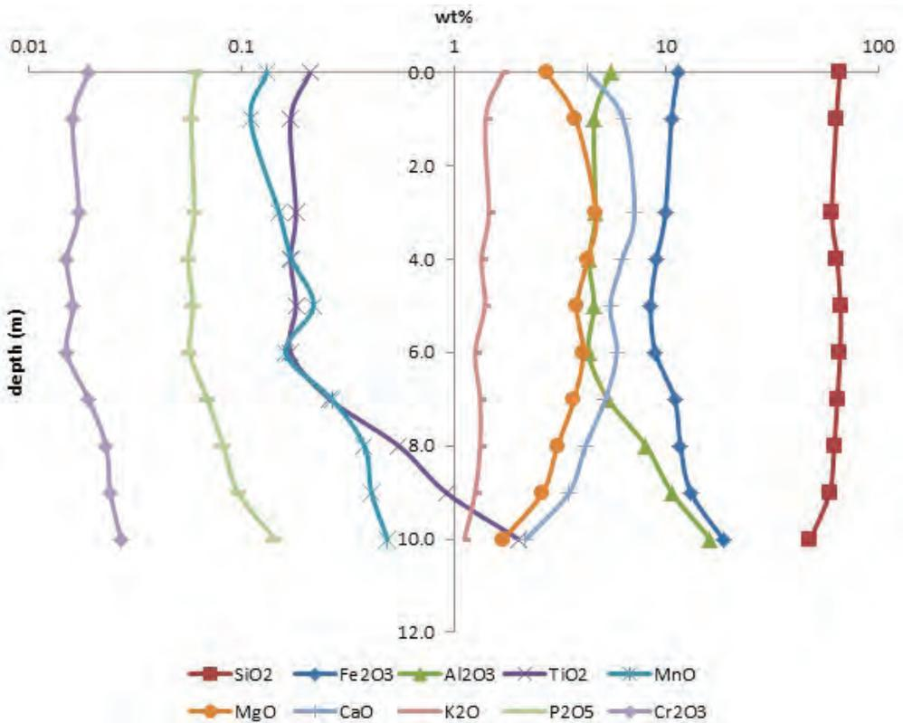
Fig. 6 Depth profile for major oxides in Glynn's Lydenburg tailings storage facility (Log 10 scale on x-axis)
