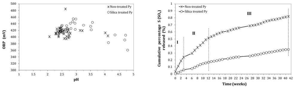
Figure 3 (a) ORP versus pH and (b) cumulative percentage of  $S(SO_4)$  released (%) vs. time in the leachates of treated and non-treated Py.
