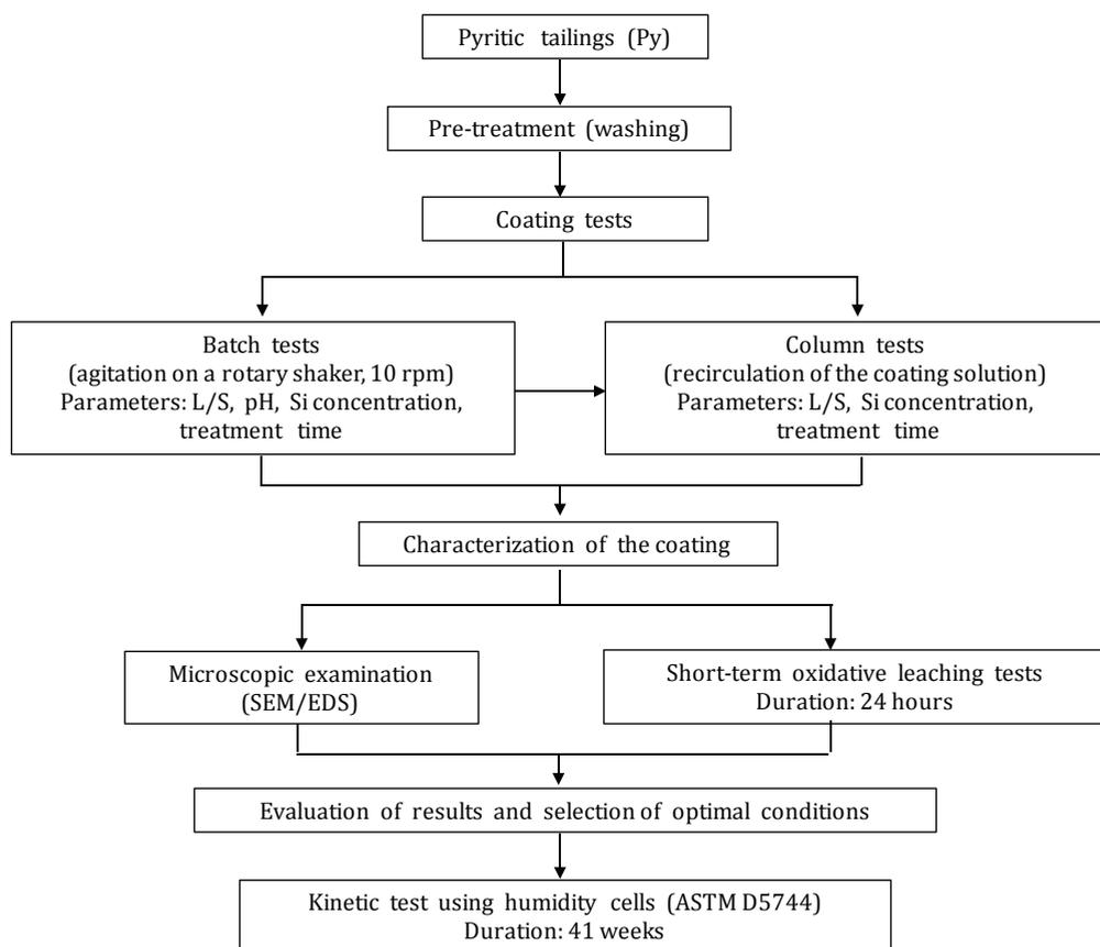
**Figure 1** Methodology used for the development of silica coating on pyrite surface and the evaluation of coating effectiveness.
