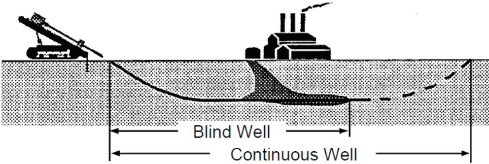
Figure 2 Horizontal well used to intercept a plume. The solid line represents a blind well; the solid line plus the dashed line represents a continuous well. (EPA, 1994).
