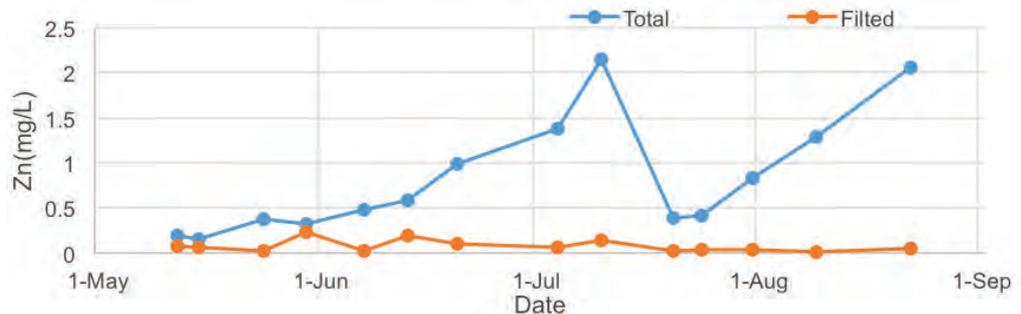
Figure 6 Changes of zinc concentration of raw water and treated water
