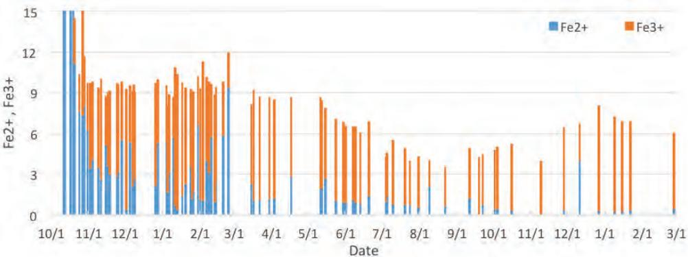
Figure 2 Changes of iron concentration of treated water
