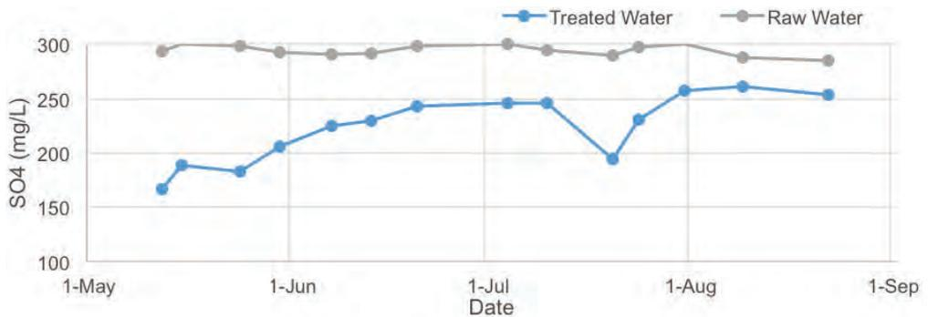
Figure 5 Changes of sulfate ion concentration of raw water and treated water
