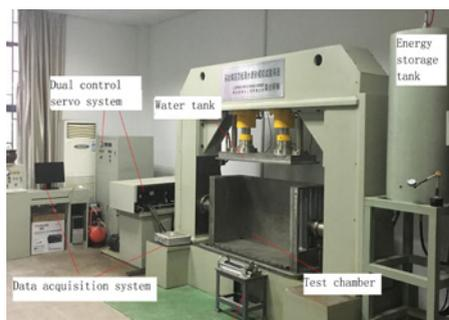
**Fig.3** Roof water and sand inrush of mining simulation system
