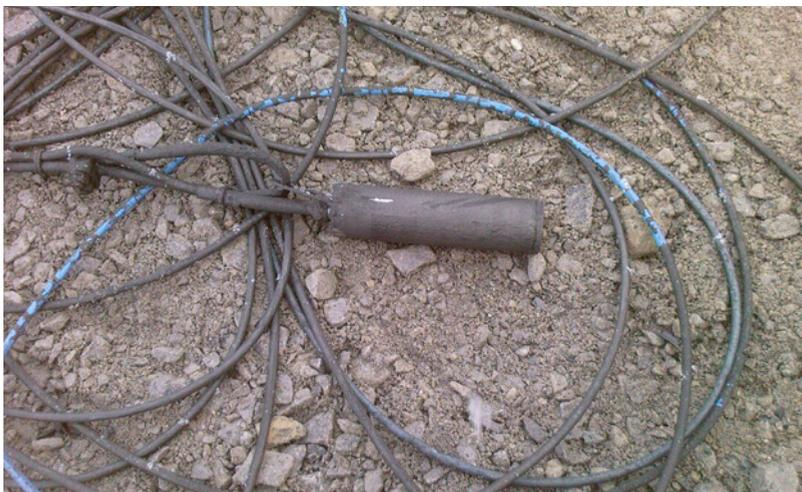
**Figure 2:** Example of stational probe for mine water level observation – recovered to surface.
