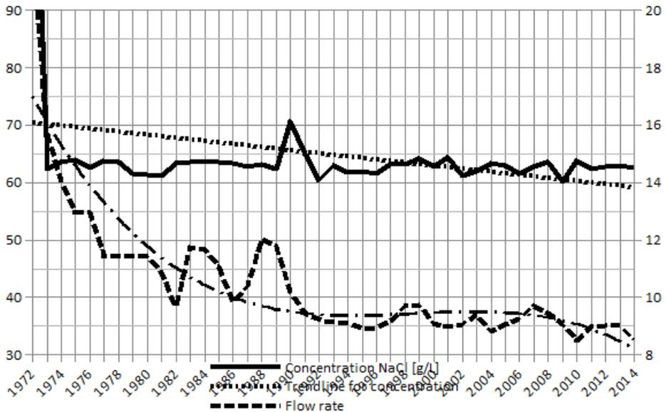
**Figure 3** Trends in the leak WVII-16 flow rate and the NaCl concentration in years 1972–2014 (own work).
