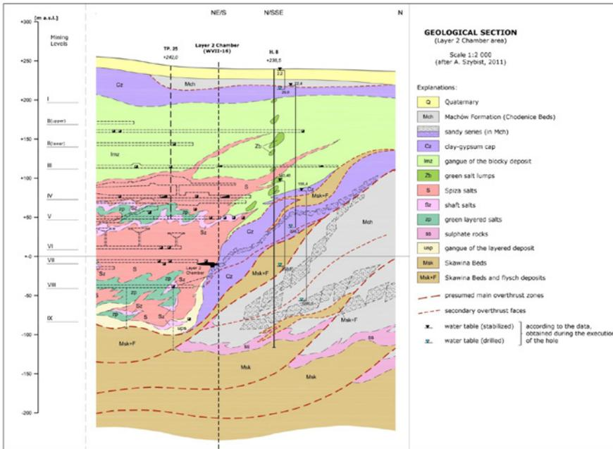
Figure 2 Geological section of the Wieliczka salt deposit in the near of the Layer 2 Chamber (after Szybist, 2011)
