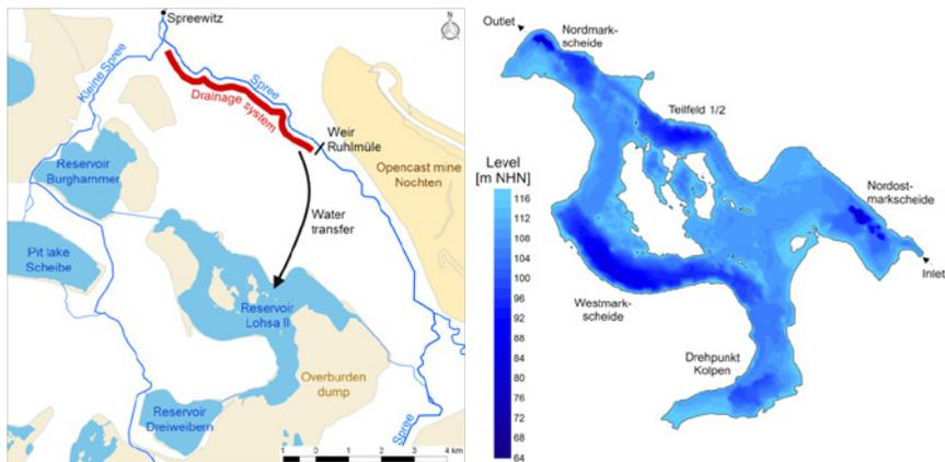
**Figure 1:** Overview of the Lohsa II reservoir system (left) and the bathymetry of the pit lake Lohsa II (right)
