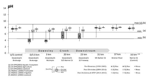
Figure 4 Progressive improvements on pH values as one of the main indicators of water quality (\*\* tributary control 16km downstream, data source: Brukunga water monitoring reports)
