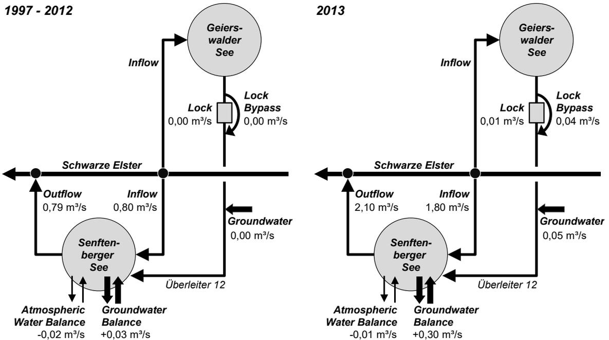
**Figure 3:** Average water balance of the Senftenberger See for the years 1997 to 2012 (left) compared with the year 2013 (right)
