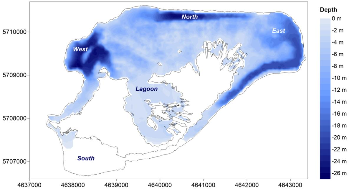
**Figure 2:** Water depths in the lake Senftenberger See at a water level of +99.25 mNHN
