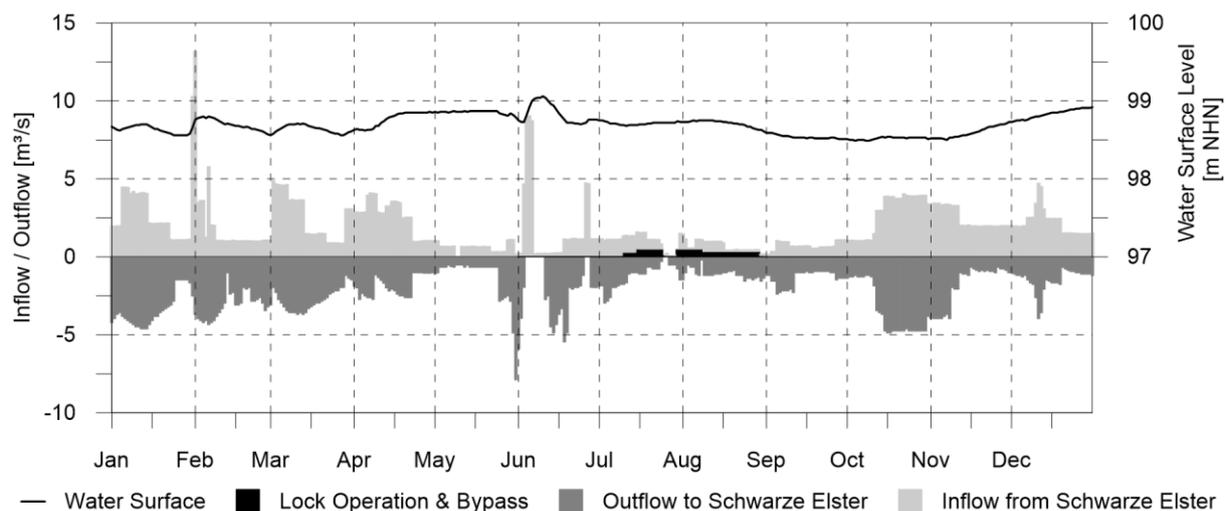
Figure 4: Surface water balance of the Senftenberger See in the year 2013
