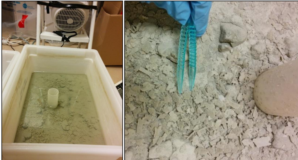
Figure 1 Bench-scale experimental tailings pond (left) and precipitate on top of dry pond (right)
