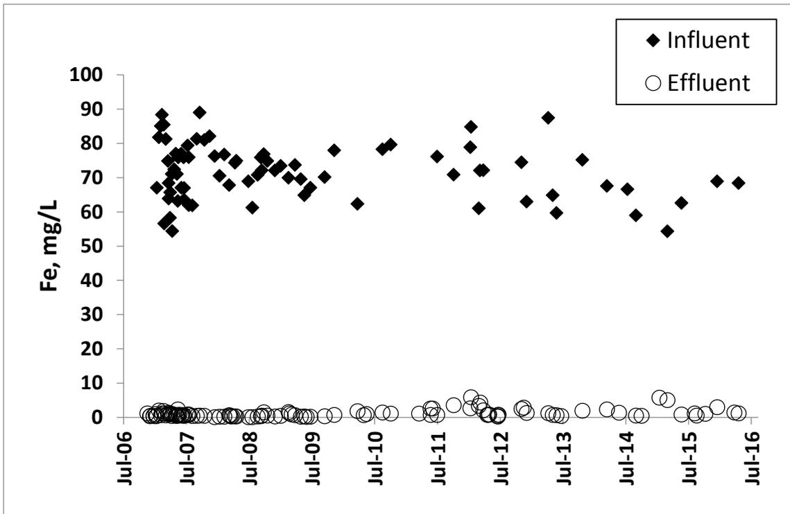
Figure 1 Influent and effluent concentrations of Fe for the Marchand passive treatment system;
