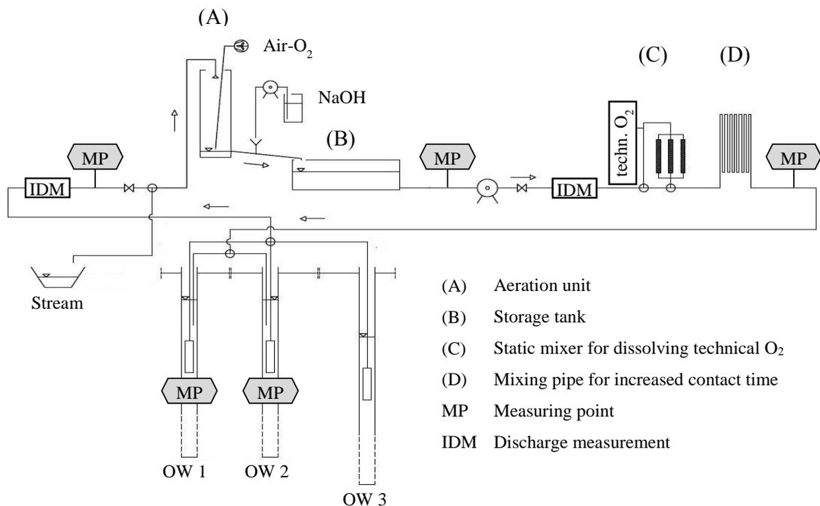
**Figure 1** Schematic of field test set-up.
