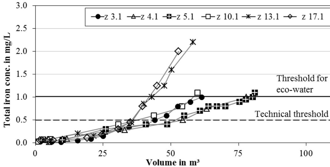
Figure 3 Iron concentrations in extracted water from OW 2 in cycles with technical oxygen.
