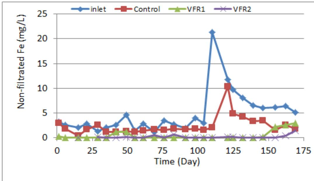
Figure 1 Comparison of non-filtered iron concentration in inlet and effluents
