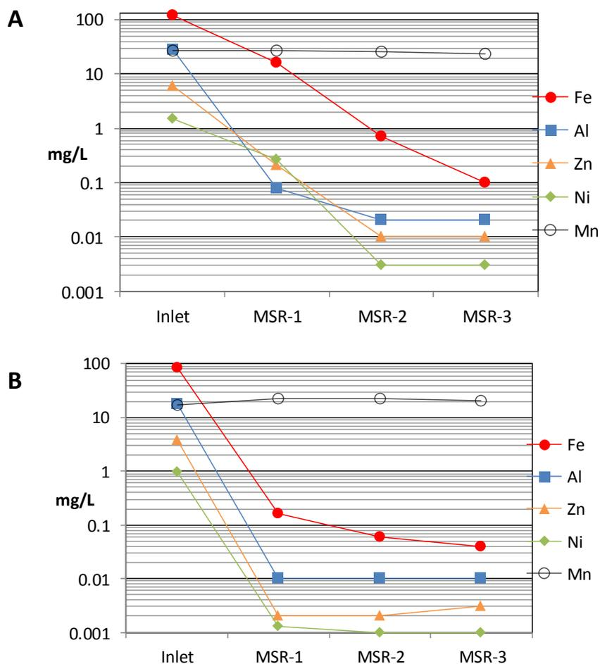
**Figure 2** Concentrations of metals through treatment system. **A** HRT of 28 hours. **B** HRT of 95 hours. MSR-1, mussel shell reactor 1; MSR-2, mussel shell reactor 2; MSR-3, mussel shell reactor 3
