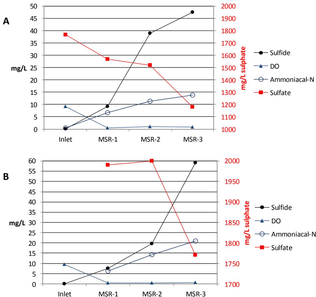
**Figure 3** Sulfur species, DO, and ammoniacal nitrogen through treatment system. **A** HRT of 56 hours. **B** HRT of 95 hours. MSR-1, mussel shell reactor 1; MSR-2, mussel shell reactor 2; MSR-3, mussel shell reactor 3
