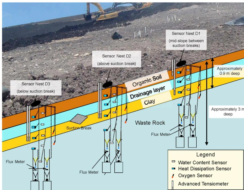
Figure 1 Cross-section of North Panel monitoring nest installation
