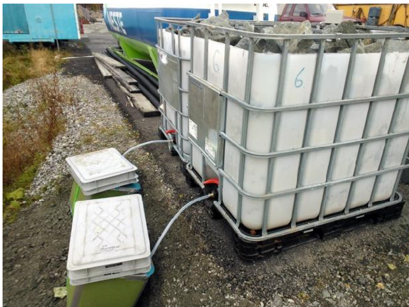
Figure 2 The aging test units 1 (front) and 2 (behind). The rain water flowing through the units was collected in the green plastic tanks below. Photo: Lauri Solismaa / GTK
