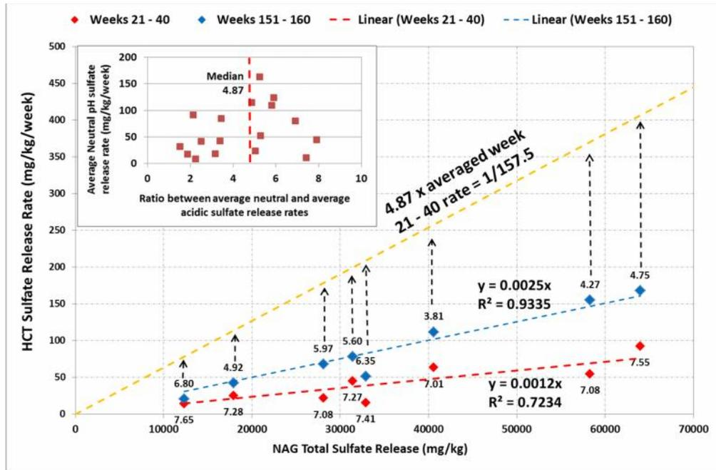
**Figure 1** Variation between NAG release (mg/kg) and HCT sulfate release rate (mg/kg/week) for weeks 21 to 40 and weeks 151 to 160 HCT data respectively. Data point labels correspond to the average HCT pH for the period. The orange dashed line corresponds to 4.87 times multiplication of the weeks 21 to 40 slope rate resulting in a slope of 1/157.5. The inset graph shows the range of ratios between sulfate release rates under neutral and acidic conditions from previous HCT data.
