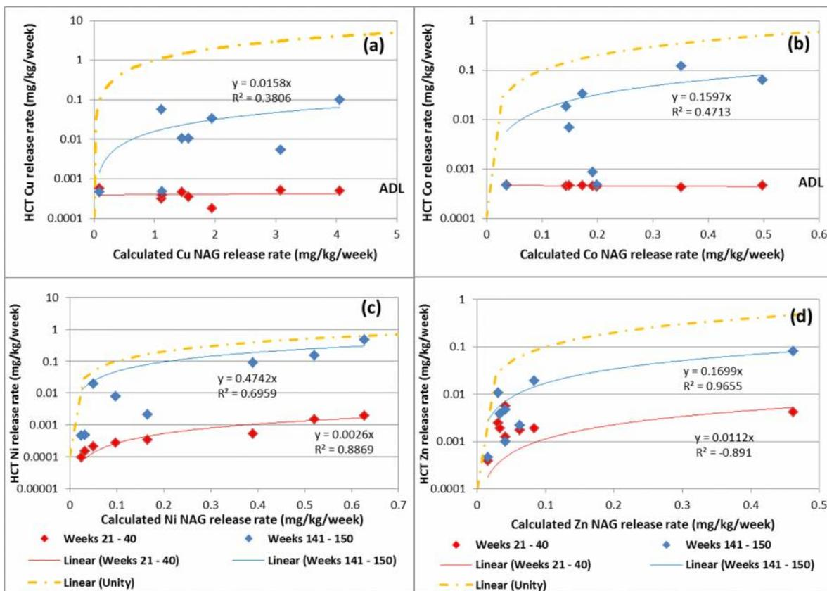
**Figure 2** Comparison between measured HCT metals release rate (mg/kg/week) and calculated NAG release rate using the factor of 157.5 correction (as mg/kg/week equivalent) for a) Cu b) Co c) Ni and d) Zn. Comparison is made for HCT weeks 21 to 40 data and HCT weeks 141 to 150 data. The orange dashed shows 1:1 ratio between measured HCT release rates and calculated NAG release rates.
