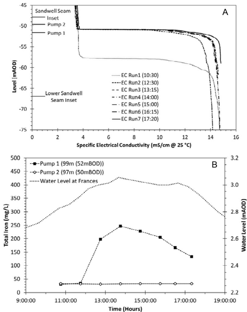
**Fig. 2** A) Graph of on-site total iron concentrations and water level at Frances, 2012. B) Electrical conductivity-temperature logs at Frances shaft, 2012
