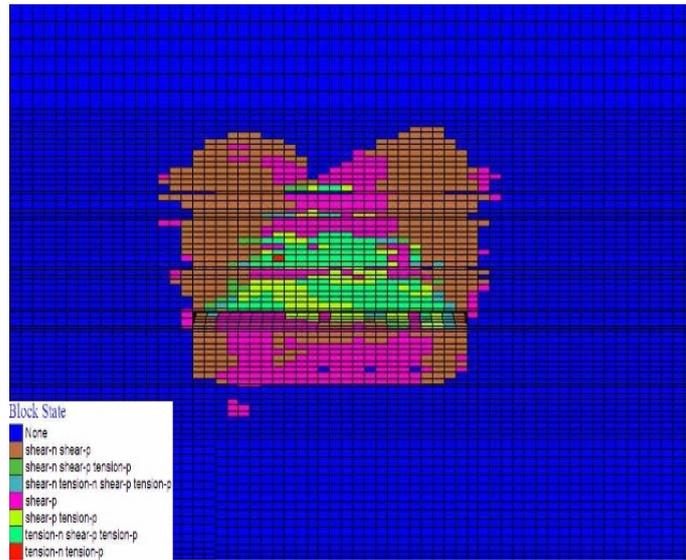
Fig.4 Cloud chart of plastic failure at 120 m in work in working face
