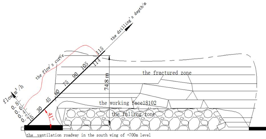
**Fig. 1** Water inflow observation in borehole on working face 18102 roof
