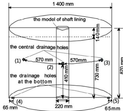
Fig.1 The size of shaft lining model equipment
