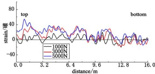
**Fig.6** Circumferential deformation of fine sand layer 40 cm away from the shaft lining under load
