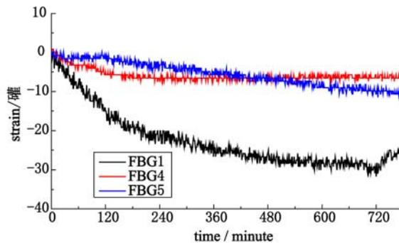
**Fig.7** Dependent variable of fine sand layer along with variation of time under water loss
