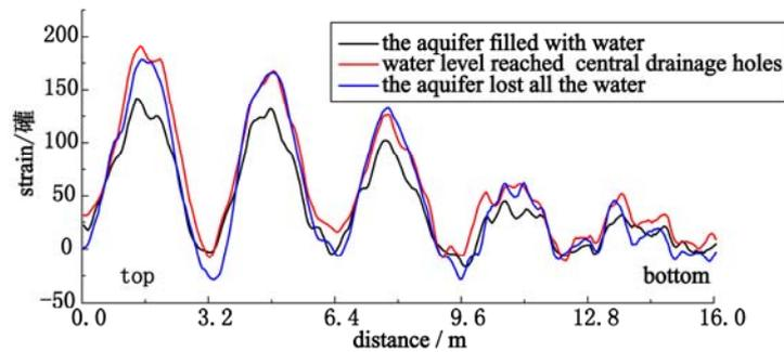
*Fig.8 Circumferential deformation of fine sand layer 40cm away from the shaft lining under water loss*
