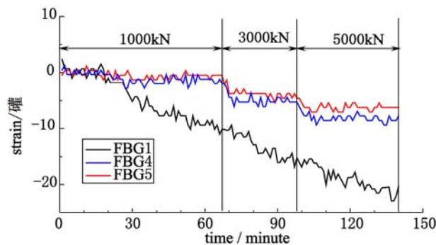
Fig.5 Dependent variable of fine sand layer along with variation of time under load
