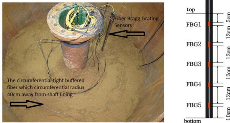
(a) The layout method of optical fiber sensors (b) The size of FBG optical fiber grating sensors
