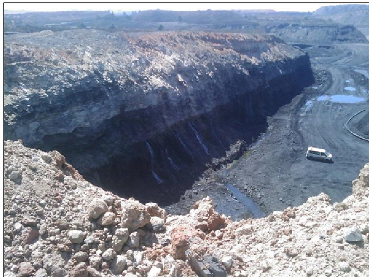
*Fig. 4 Seepage from the high wall*
