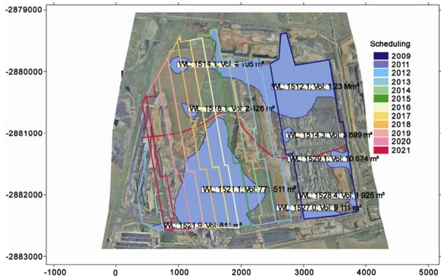
Fig. 2 Water in the opencast at 1512.10 mamsl (watershed line and scheduling superimposed)
