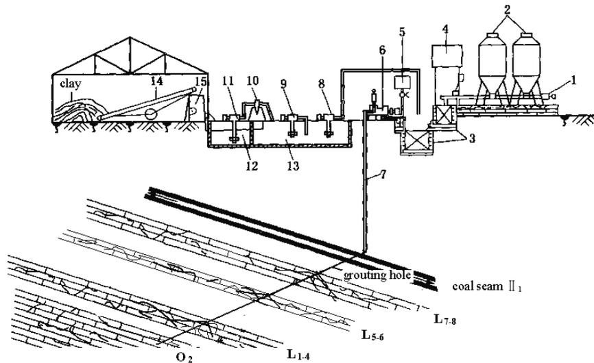
**Fig. 1** The diagram of the floor consolidation grouting system
