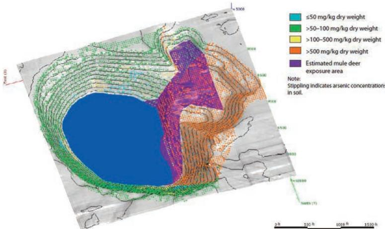
*Fig. 1 Predicted pit-lake geometry and arsenic distribution in the Vista Pit.*
