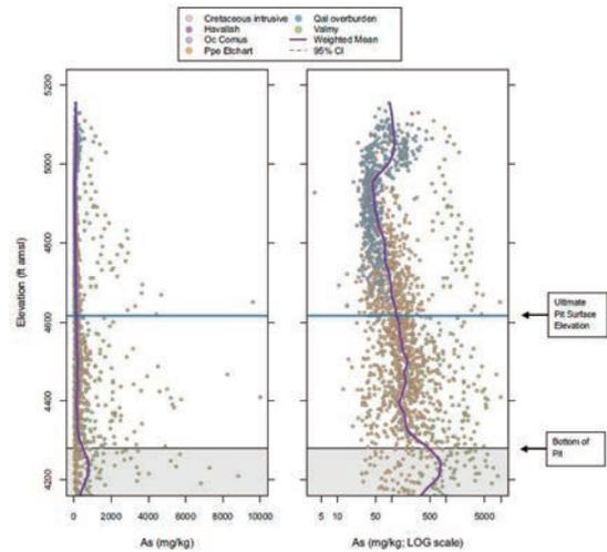
**Fig. 2.** Arsenic concentrations as a function of depth in the proposed Vista Pit.
