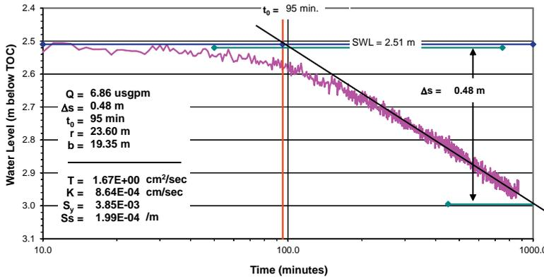
**Fig. 3** Pumping Test Observation Data Analysis-Jacob Straight Line Method
