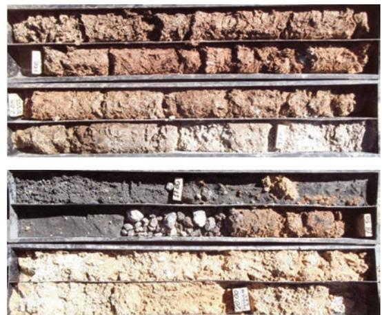
Fig. 2 Pictures of typical bofedal drill core.
