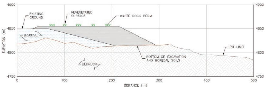
Fig. 5 Cross section of buttress required to support bofedal slope
