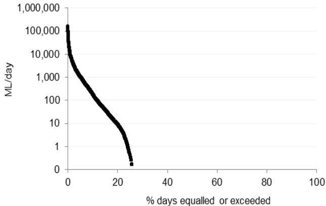
**Figure 2** Exceedance curve of stream flow in the Isaac River at Deverill (data: DNRM 2012).
