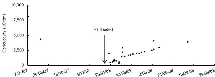
**Figure 4** Electrical conductivity of water stored in a flooded mine pit in the Bowen Basin during the 2007-08 wet season.
