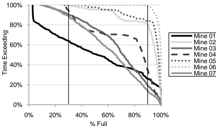
**Figure 3** Water status of seven mine sites in the Bowen Basin. Wet and dry indicators are shown by the vertical solid lines. One site has a high risk of running dry (black solid line) while two other sites have a significant risk of requiring to discharge being >90% full at least 80% of the time (Moran et al. 2006).
