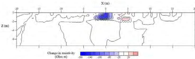
**Figure 14** Changes in the modelled resistivity values (as compared to the background values) along the west/east profile 3130 min (52 hr, 10 min) after brine injection commenced (2850 min after removal of constant head).
