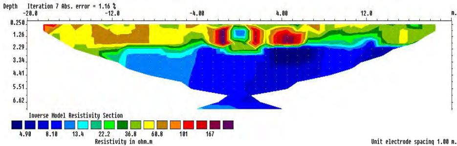
**Figure 8** Constant head resistivity measurement after 1 hour and 8 minutes.
