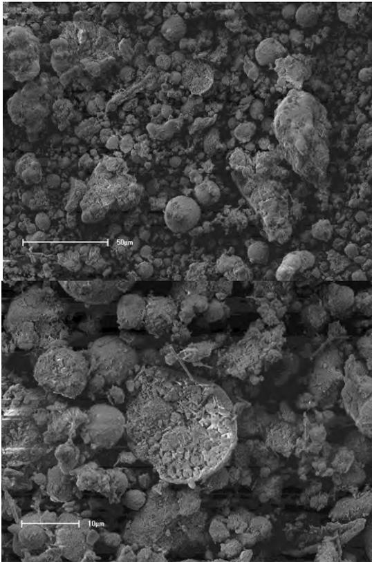
**Figure 2** Scanning electron microscopy (SEM) photos of industrial fly ash at 50 and 10 micron meters, respectively.
