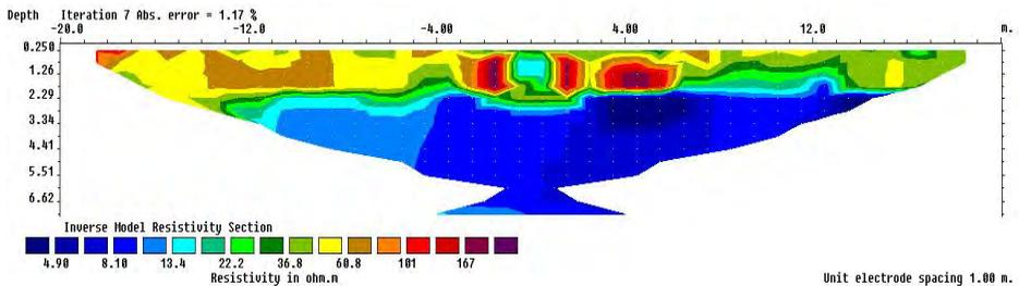
**Figure 9** Constant head resistivity measurement after 1 hour and 46 minutes.
