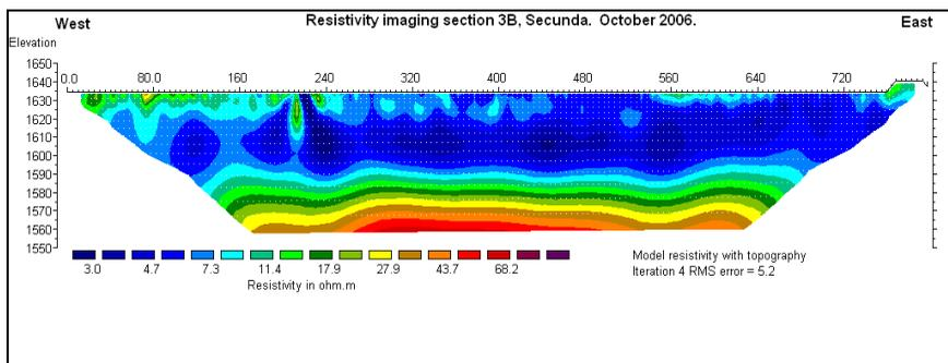
**Figure 3** Resistivity imaging of a section of the surface area of the fly ash dam.
