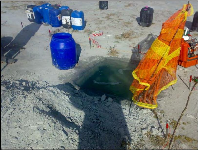
**Figure 5** Photograph of the survey setup (view towards the south-east). A constant head level with the ash surface is maintained in the injection pit during the injection phase.
