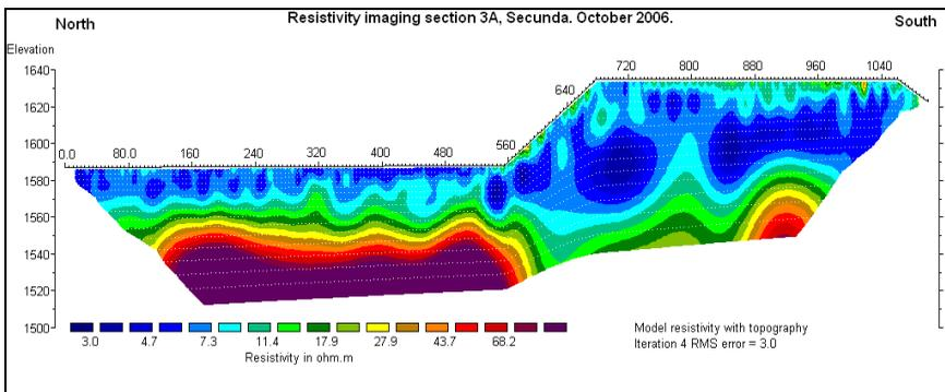
**Figure 2** Resistivity imaging of section of the surrounding area and the fly ash dump was done over a one kilometre area. On the left side of the image the surrounding area is mapped while on the right-hand side the fly ash dam influence is shown.
