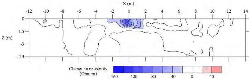
**Figure 13** Changes in the modelled resistivity values (as compared to the background values) along the north/south profile 3160 min (52 hr, 40 min) after brine injection commenced (2880 min after removal of constant head).
