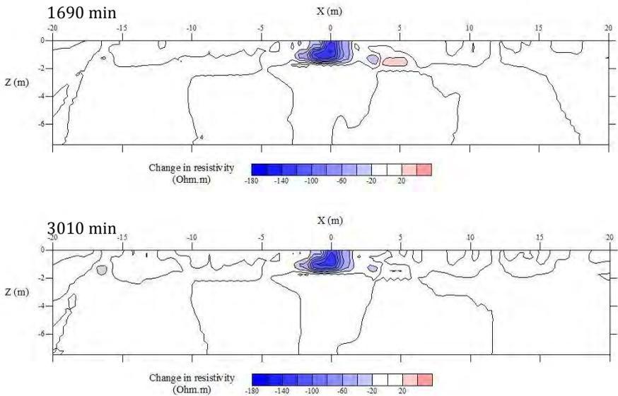
**Figure 12** Changes in the modelled resistivity values (as compared to the background values) along the west/east profile at specified time intervals after brine injection commenced and removal of constant head.
