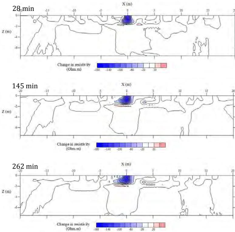
**Figure 11** Changes in the modelled resistivity values (as compared to the background values) along the west/east profile at specified time intervals after brine injection commenced (under constant head conditions).
