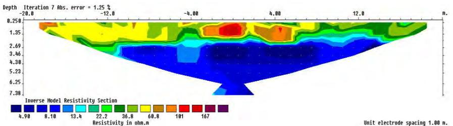
**Figure 6** Resistivity imaging of the top section of the fly ash dam. A cross-profile of the surface area of the fly ash dam is presented. A hole was dug at position 0 (centre of figure) which was 1 m x 1 m in extent and 0.5 m in depth. The impact on the resistivity measurements can be seen in this area, with an elevated resistivity reading.
