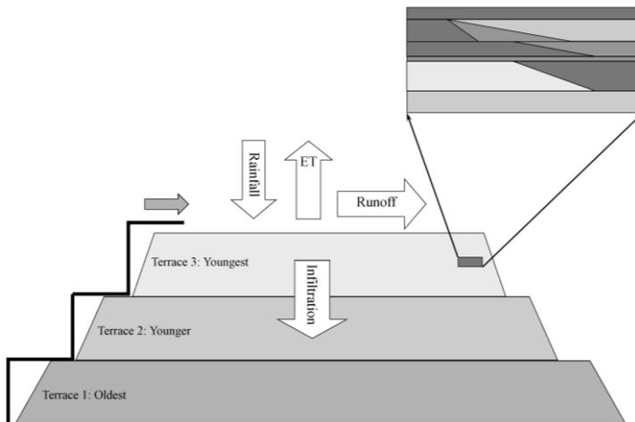
**Figure 1** Construction and initial conceptual model of fly ash dam, showing the hydrological processes.
