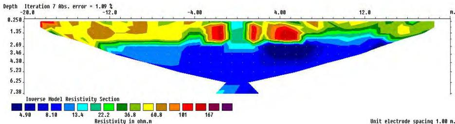
**Figure 10** Constant head resistivity measurement after 4 hours and 22 minutes.
